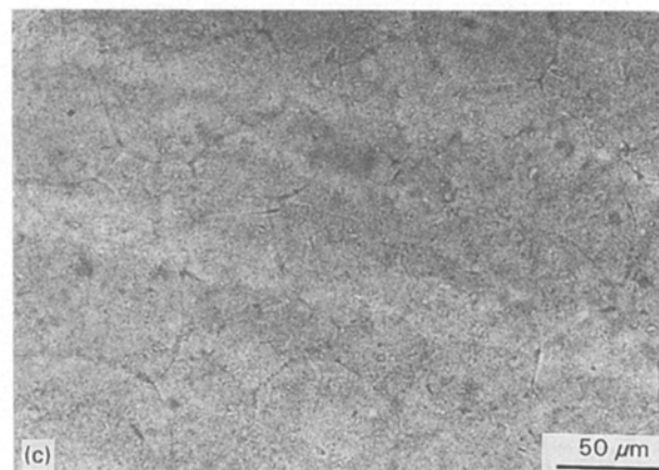
Figure 2 Optical micrographs of the compacts with various PVA contents. (a) 3.85 wt.%; (b) 2.24 wt.%; (c) 1.6 wt.%; after binder removal.
